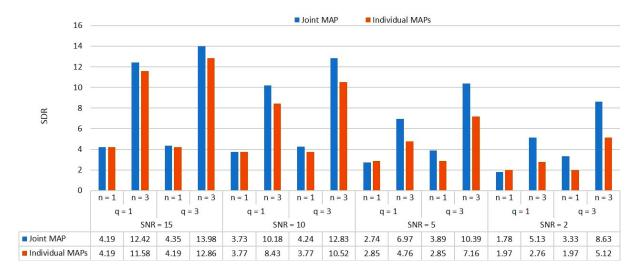
Fig. 7: Simulation SDR results (in dB) of joint MAP decoding and having two independently designed MAP decoders for two binary-quantized correlated Gaussian sources with Markovian correlation parameter. The channel model is a MAC with two orthogonal NBNDC-QB, with  $M=\alpha=1$ , Cor=Cor'=0.9 and identical parameters (SNR,q); q=1,3. Source parameters are  $\phi_{\rm av}=0.61$ ,  $\phi_0=-0.31$ ,  $\phi_1=0.81$  and  $(t_{\phi_0\phi_0},t_{\phi_1\phi_1})=(0.1,0.8)$ . SQs with n=1,3 are used.
