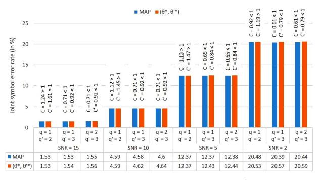
Fig. 5: Joint symbol error rate (in %) of joint MAP decoding and instantaneous joint decoding  $(\theta^*, \theta'^*)$  for two binary-quantized correlated Gaussian sources with Markovian correlation parameter. The channel model is a MAC with two orthogonal NBNDC-QB, with  $M=\alpha=1$ , Cor=Cor'=0, q=1,2,3 and identical parameter SNR. Source parameters are  $\phi_{\rm av}=0.25$ ,  $\phi_0=-0.31$ ,  $\phi_1=0.81$  and  $t_{\phi_0\phi_0}=t_{\phi_1\phi_1}=0.2$
