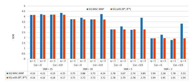
Fig. 6: Simulation SDR results (in dB) of joint MAP decoding and instantaneous joint decoding  $(\theta^*, \theta'^*)$  for two binary-quantized correlated Gaussian sources with Markovian correlation parameter. The channel model is a MAC with two orthogonal NBNDC-QB, with  $M=\alpha=1$  and identical parameters (Cor, SNR,q); q=1,3 and Cor=0,0.9. Source parameters are  $\phi_{\rm av}=0.61,\,\phi_0=-0.31,\,\phi_1=0.81$  and  $(t_{\phi_0\phi_0},t_{\phi_1\phi_1})=(0.1,0.8)$ . SQs with n=1 are used.
