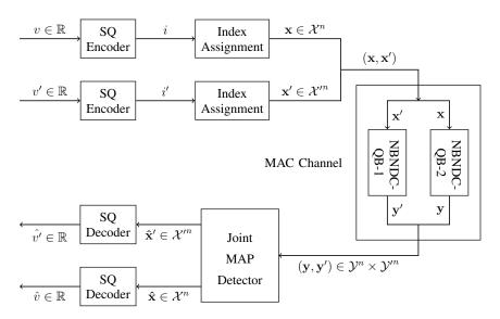
Fig. 2: Two-user system with scalar quantization and joint MAP decoding over an orthogonal MAC with memory.
