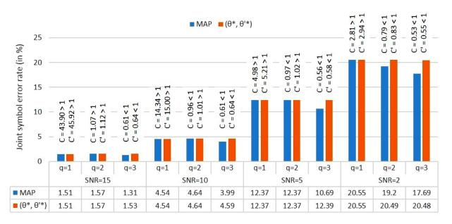
Fig. 4: Joint symbol error rate (in %) of joint MAP decoding and instantaneous joint decoding  $(\theta^*, \theta'^*)$  for two binary-quantized correlated Gaussian sources with Markovian correlation parameter. The channel model is a MAC with two orthogonal NBNDC-QB, with  $M=\alpha=1$ , Cor=Cor'=0 and identical parameters (SNR,q); q=1,2,3. Source parameters are  $\phi_{\rm av}=0.61$ ,  $\phi_0=-0.31$ ,  $\phi_1=0.81$  and  $(t_{\phi_0\phi_0},t_{\phi_1\phi_1})=(0.1,0.8)$
