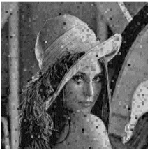
Decoded Lena with \delta = 0.0 , \epsilon = 0.1 , PSNR = 22.67 dB
