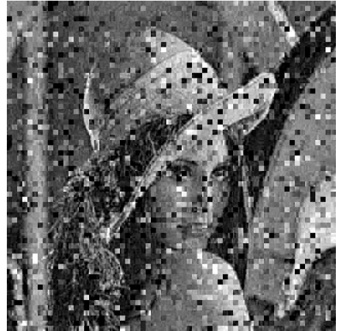
Decoded Lena with SQ-IL, PSNR = 15.84 dB
