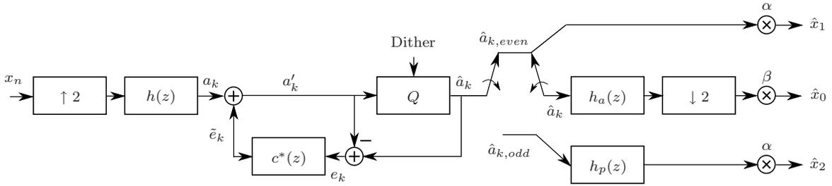
Figure 2.11: Delta-Sigma quantization scheme with two channels.
