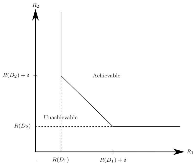
Figure 2.3: Achievable rates for multiple description coding of a unit variance memoryless Gaussian source with squared-error distortion. The minimum excess rate  $\delta$  is a function of  $(D_0, D_1, D_2)$  and may be zero.
