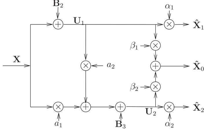
Figure 2.8: MD successive quantization scheme for  $V_1$ .
