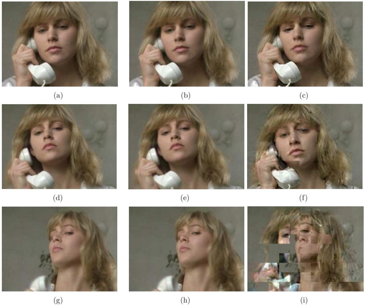
Figure 5.3: Effect of loss of motion vectors and loss of the same amount of prediction error bits on MPEG video Suzie. Frames on the left are the originals, motion vectors of frames on the right are lost, and the same number of prediction error bits in each frame in the middle column is lost too. (a),(b),(c) Frame No. 51. (d),(e),(f) Frame No. 87. (g),(h),(i) Frame No. 107.
