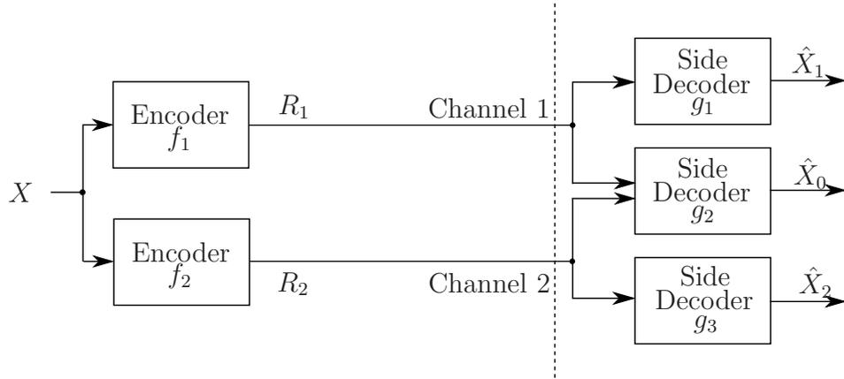
Figure 2.5: Multiple description scalar quantizer with two channels.
