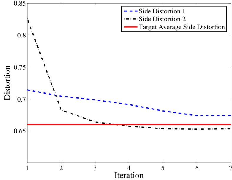
Figure 3.2: Effect of tuning the Lagrangian multipliers on side distortions for a memoryless Gaussian input source and target side distortions  $D_{1,t} = D_{2,t} = 0.66$ .  $k = 4$ , and  $R = 0.5$  bps.
