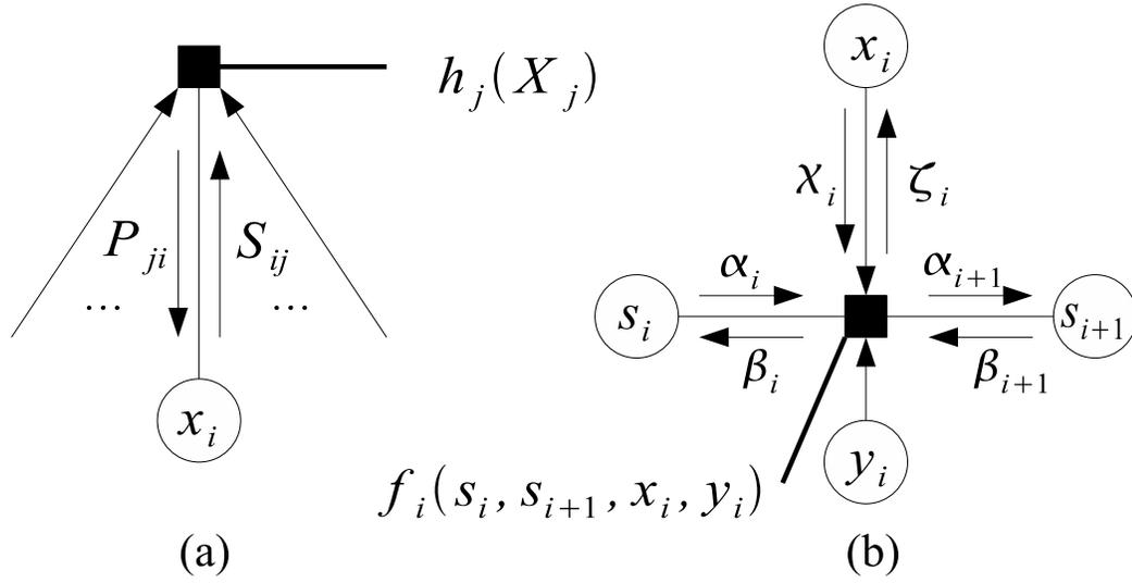
Figure 4.3: Graphs showing the messages and factor nodes associated with the parity-check factors (a) and the channel factors (b).
