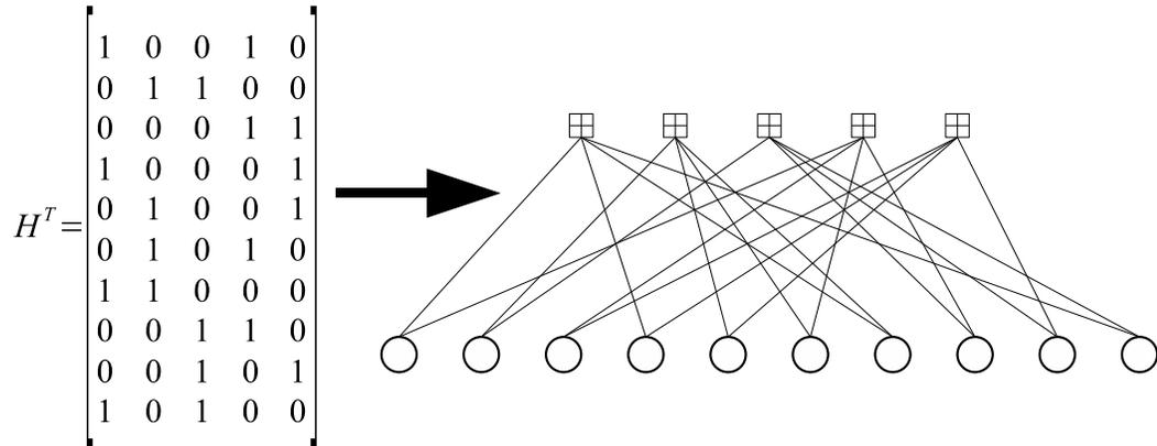
Figure 3.2: Example of a length 10 (2,4)-regular LDPC code in both parity-check and Tanner graph forms.
