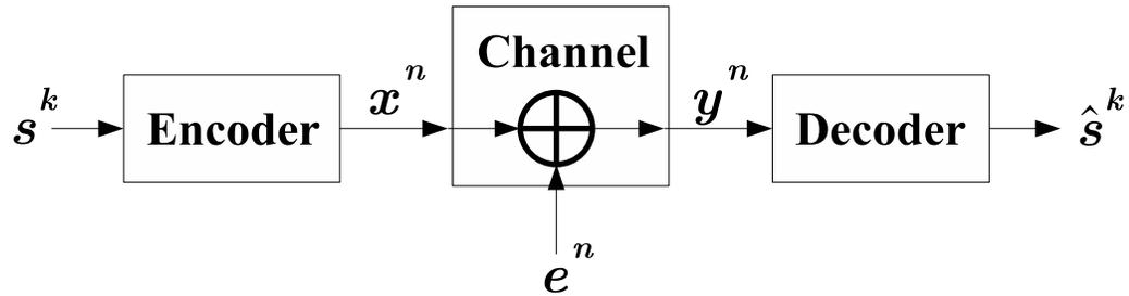
Figure 4.1: Block diagram of an error-correcting coding communication system with an additive noise channel.
