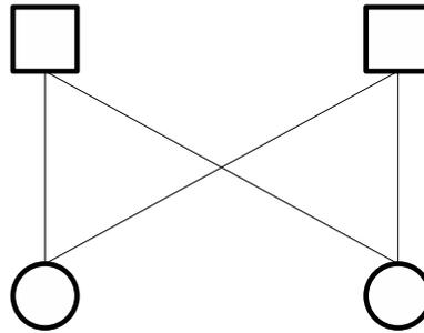
Figure 3.3: Example of a length 4 cycle in a Tanner graph.
