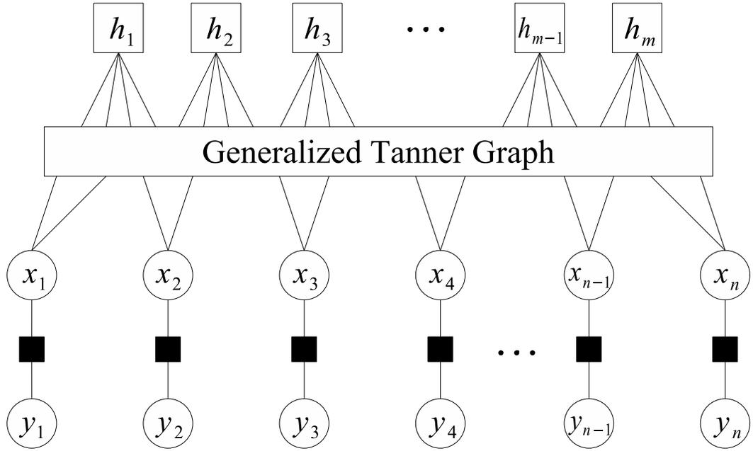
Figure 3.8: Factor graph of (3.15) for decoding parity-check codes over memoryless channels.
