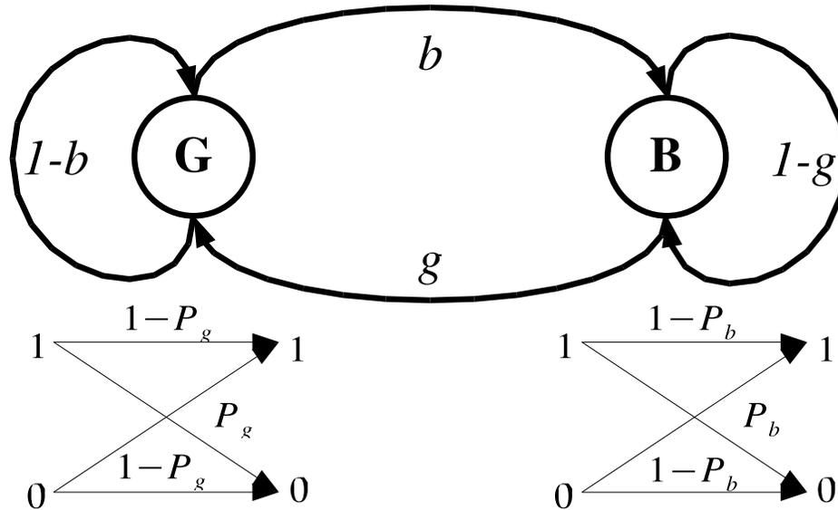
Figure 2.2: Finite state machine model for the GEC
