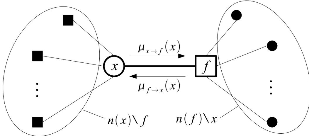
Figure 3.7: The messages passed between variable nodes and factor nodes by the SPA from Def'n. 3.2.2.
