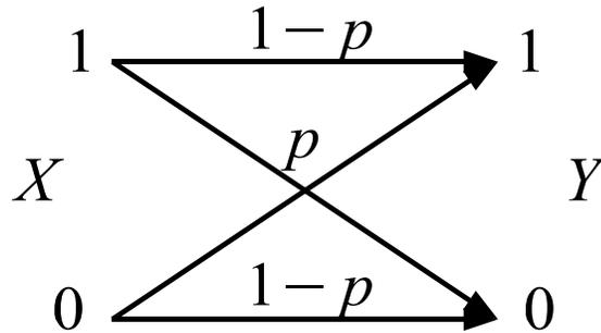
Figure 1.2: Channel transition diagram for the BSC.
