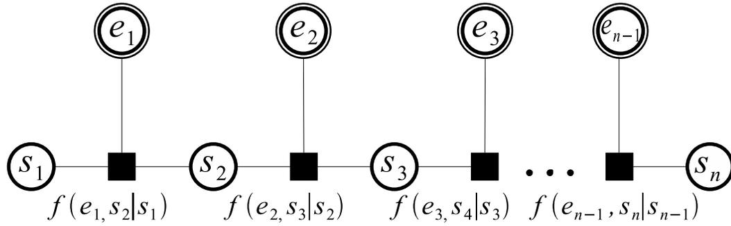
Figure 3.6: A factor graph for the state-sequence of a hidden Markov model (Wiberg-type graph).
