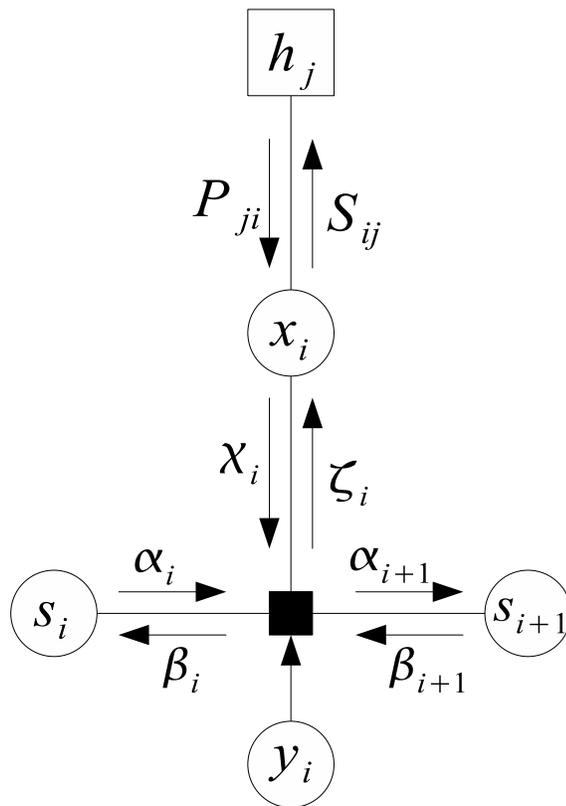
Figure 3.10: All the local messages passed for the extended SPA decoder
