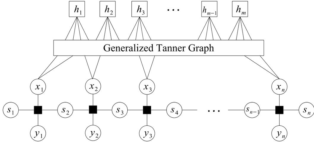
Figure 3.9: Factor graph of (3.16) for decoding parity-check codes over finite-state Markov channels.
