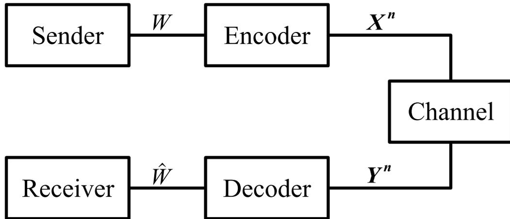
Figure 1.1: Diagram of a basic communication system utilizing an encoder and decoder to correct errors.
