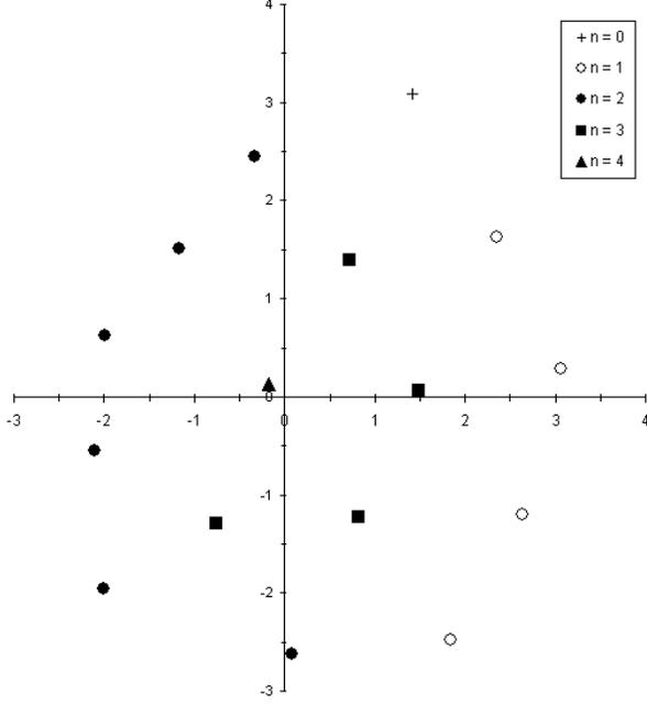
**Figure 2. Pairwise optimized constellation for  $M = 16$ ,  $p = 0.9$  and design SNR = 1 dB.**
