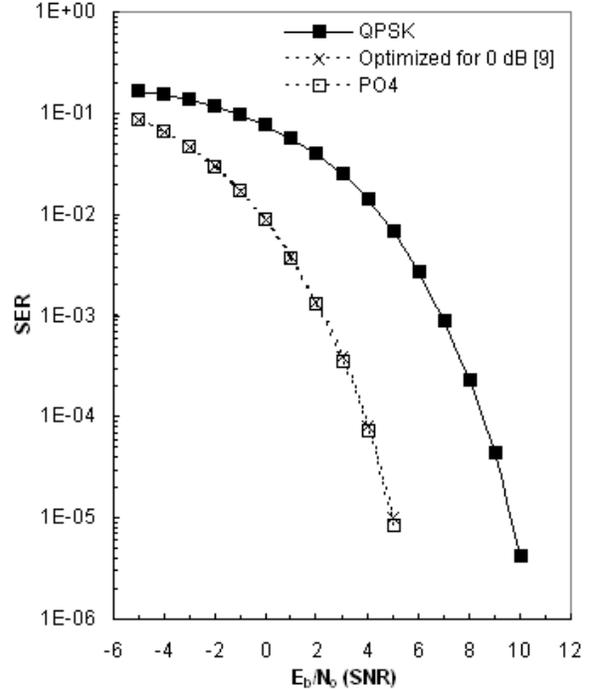
**Figure 1. Performance of  $M = 4$  constellations for  $p = 0.9$ . Optimized from [9] and PO4 are both designed for SNR = 0 dB.**
