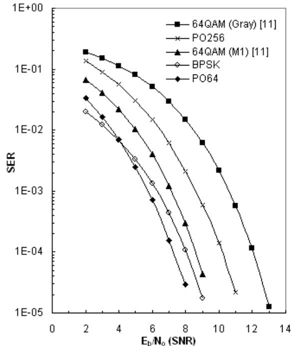
**Figure 5. Performance of constellations for  $M = 64$ ,  $p = 0.9$  and design SNR = 2 dB and the pairwise optimized constellation for  $M = 256$  with design SNR = 4 dB. BPSK also shown as reference point.**
