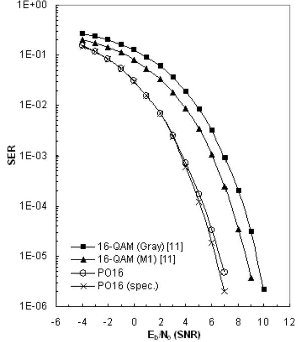
**Figure 3. Performance of  $M = 16$  constellations for  $p = 0.9$  and design SNR = 1 dB. Performance of a specialized constellation (i.e., with design SNR identical to true SNR) also shown.**
