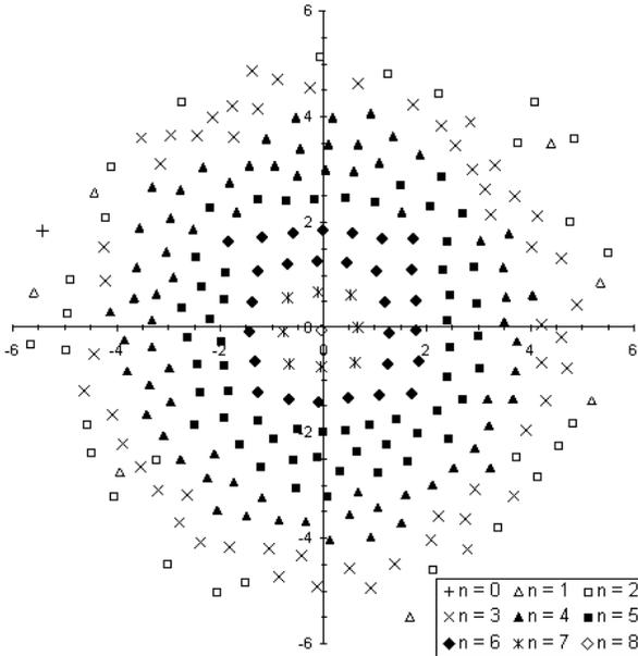
**Figure 6. Pairwise optimized constellation for  $M = 256$ ,  $p = 0.9$  and design SNR = 4 dB.**
