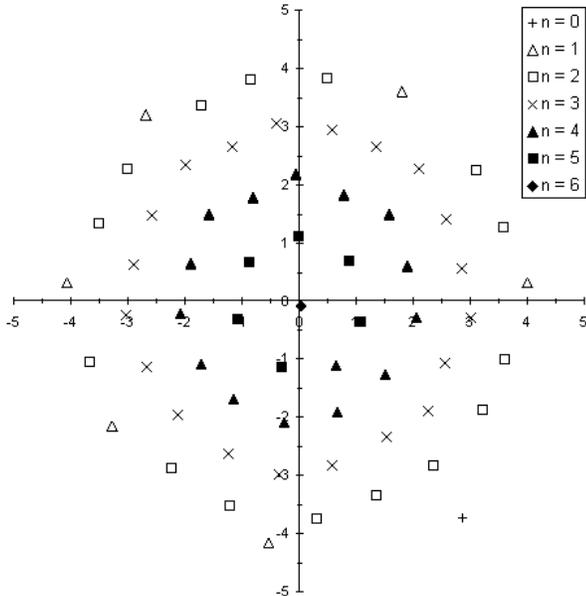
**Figure 4. Pairwise optimized constellation for  $M = 64$ ,  $p = 0.9$  and design SNR = 2 dB.**
