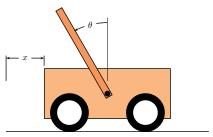
The input is a horizontal force applied to the cart.
