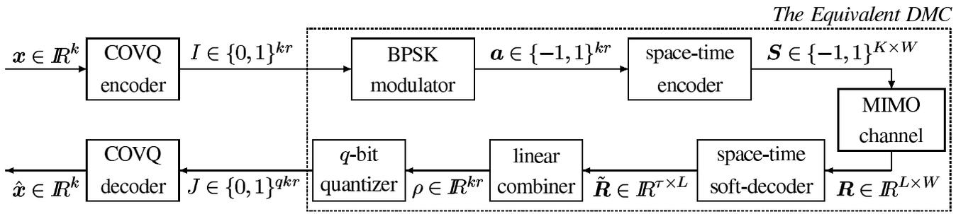
Fig. 1. System block diagram, where every  $\tau$  bits in a  $kr$ -bit index  $I$  is transmitted via a space-time codeword  $\mathbf{S}$ , received as  $\mathbf{R}$ , and space-time soft-decoded as  $\tilde{\mathbf{R}}$ . For simplicity, we have assumed here that  $\tau = kr$ .
