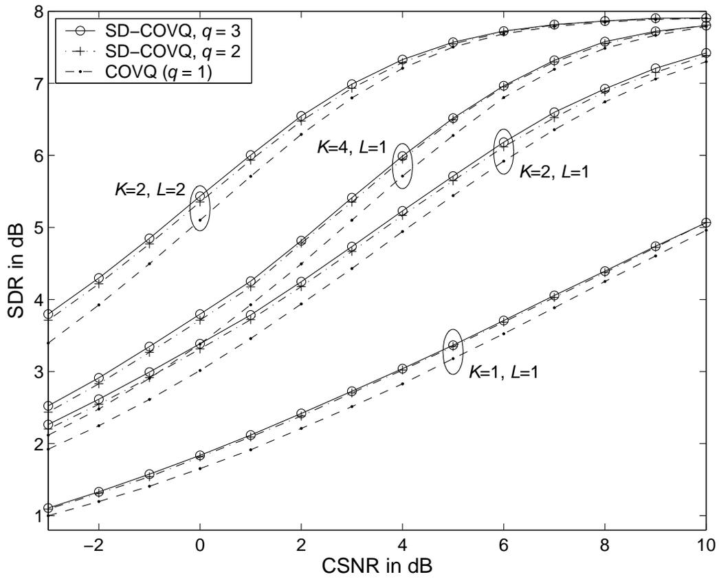
Fig. 3. Simulated SDR in dB for a zero-mean unit-variance Gauss-Markov source ( $\rho = 0.9$ ) vector quantized at rate 1 bps and soft-decision decoded with  $q$  bits. Quantization dimension is 2.
