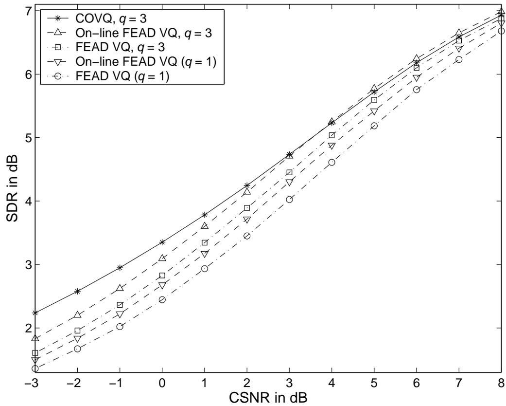
Fig. 6. Comparison among the COVQ, FEAD VQ, and On-line FEAD VQ for a  $\mathcal{N}(0, 1)$  Gauss-Markov source vector quantized at rate 1.0 bps and hard decoded. Quantization dimension is 2,  $K = 2$ , and  $L = 1$ .
