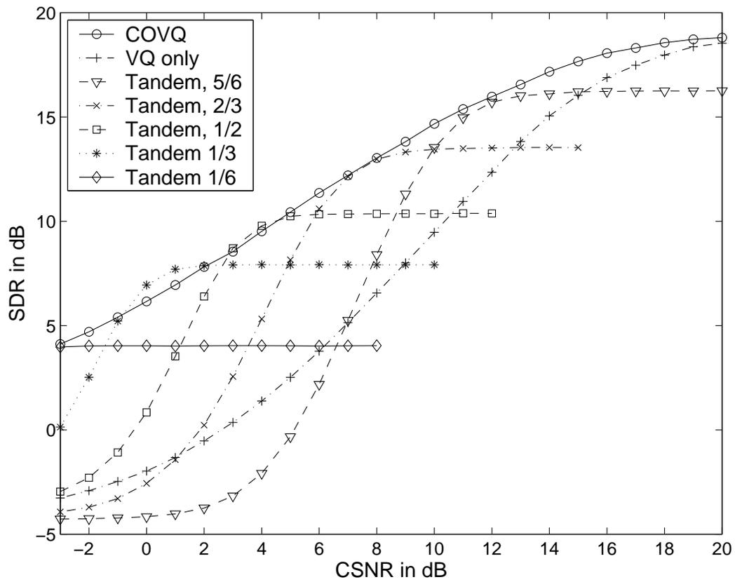
Fig. 4. Jointly designed versus tandem coding schemes for a zero-mean unit-variance Gauss-Markov source ( $\rho = 0.9$ ). Quantization dimension is 2 and the overall rate is 3.0 bps.  $K = 2$  and  $L = 1$ .
