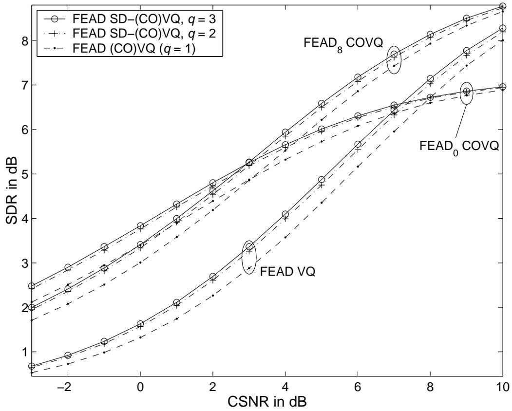
Fig. 5. Simulated SDR in dB for an i.i.d.  $\mathcal{N}(0,1)$  source vector quantized at rate 2.0 bps and soft-decision demodulated with  $q$  bits. Quantization dimension is 2.  $K = 2$  and  $L = 1$ .
