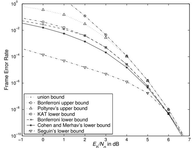
Figure 3: Frame error rate bounds for BCH (63, 24) code, BPSK signaling, and AWGN channel.
