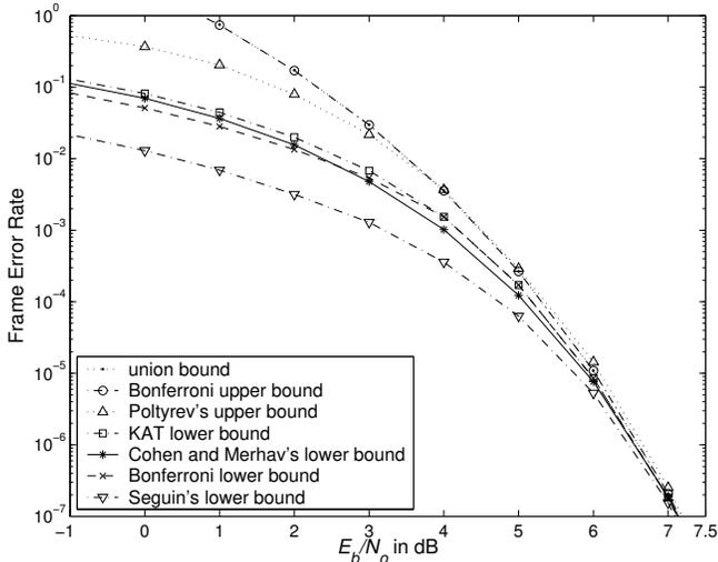
Figure 2: Frame error rate bounds for Golay (23, 12) code, BPSK signaling, and AWGN channel.
