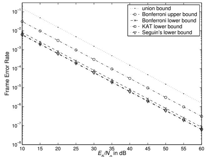
Figure 5: Frame error rate bounds for BCH (15, 5) code, BPSK signaling, and Rayleigh fading channel.
