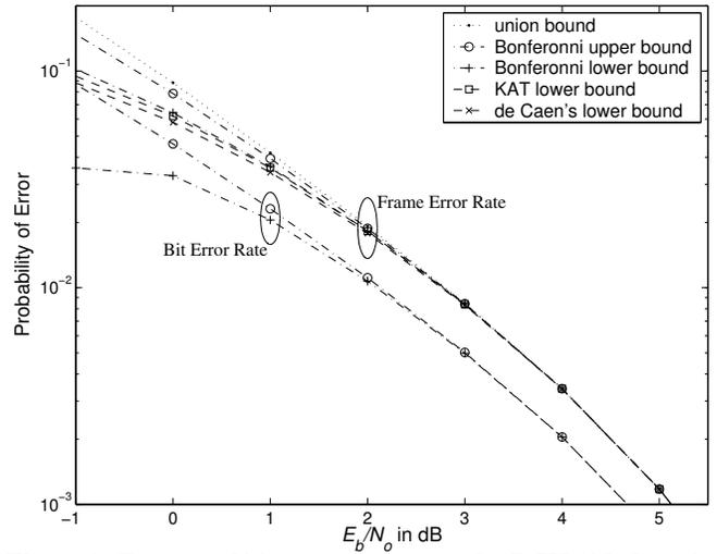
Figure 1: Frame and bit error rate curves for BCH (15, 5) code, 8-PSK modulation, and AWGN channel.
