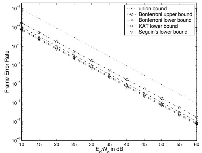
Figure 4: Frame error rate bounds for Hamming (7, 4) code, BPSK signaling, and Rayleigh fading channel.
