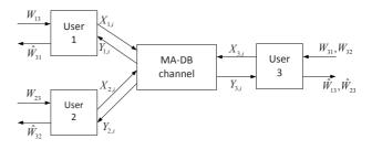
Fig. 2. Multiple access/degraded broadcast channel.
