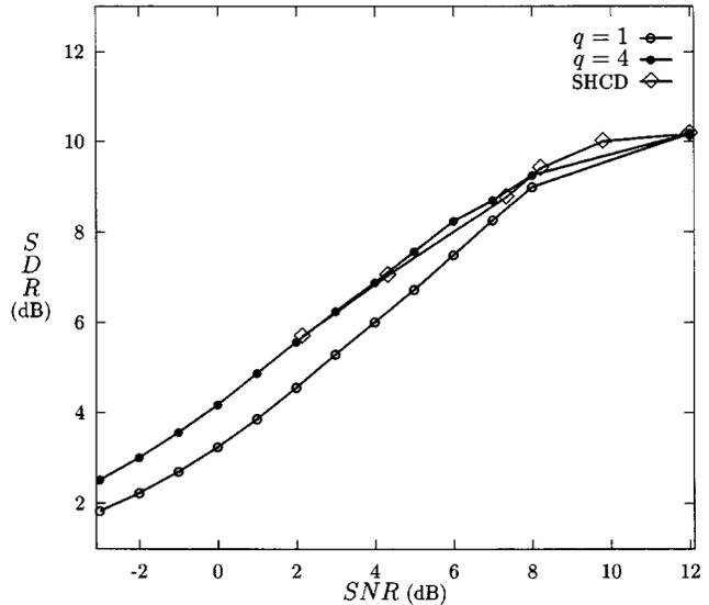
Fig. 2. Performances of COVQ system in AWGN channel with  $q = 1$  and  $q = 4$  compared with SHCD (cf. [18, Table 4]). Gauss-Markov source.  $R = 1$ ;  $k = 4$ .
