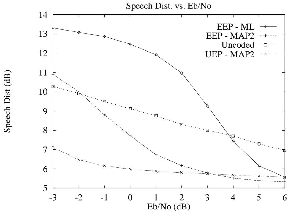
Figure 9: Average Speech Distortion for Different Coding Schemes of all the CELP Parameters over the Rayleigh Fading Channel.
