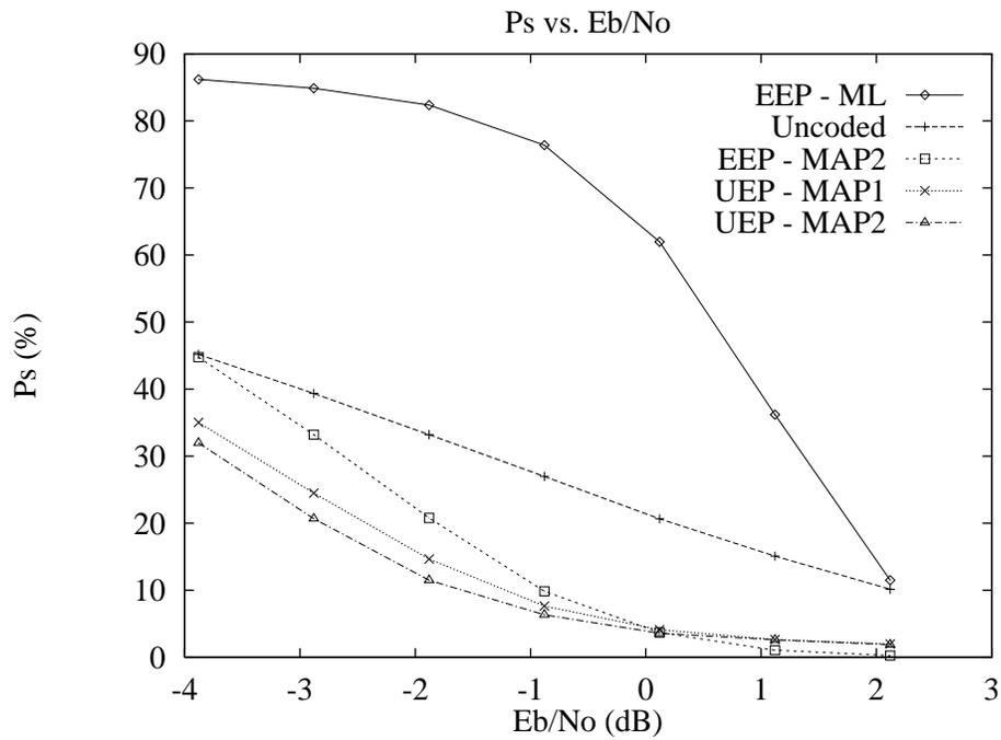
Figure 5: Symbol Error Rates for Different Coding Schemes of the LSP Parameters over the AWGN Channel.
