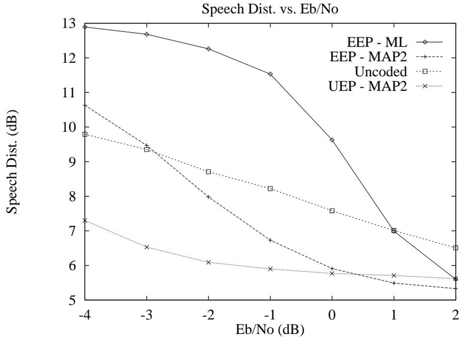
Figure 8: Average Speech Distortion for Different Coding Schemes of all the CELP Parameters over the AWGN Channel.
