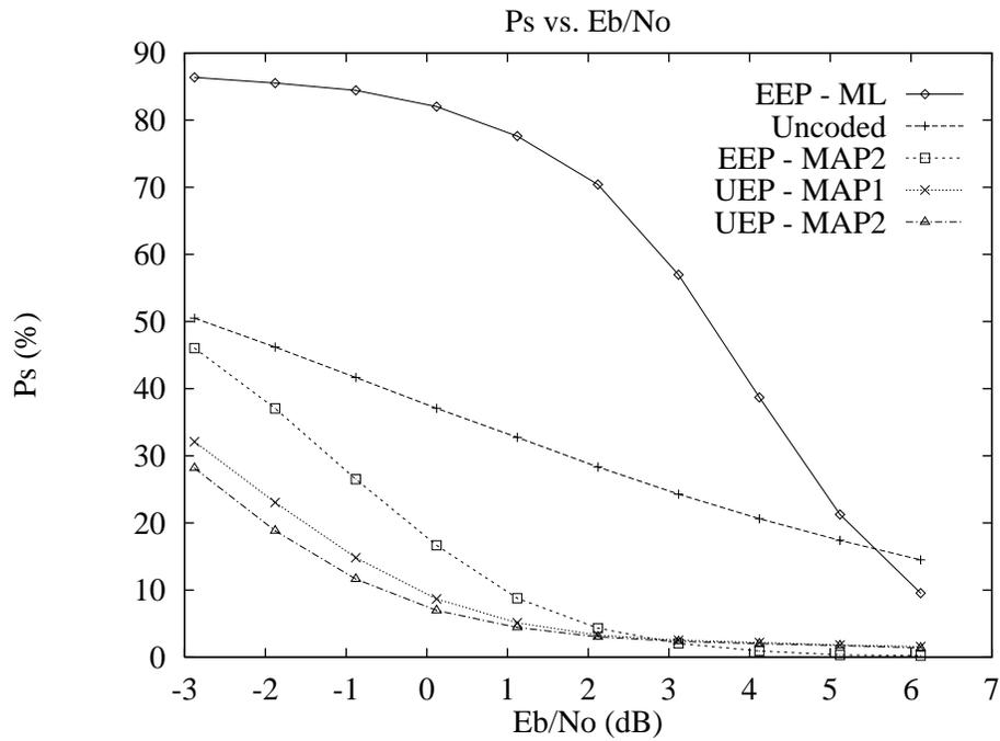
Figure 7: Symbol Error Rates for Different Coding Schemes of the LSP Parameters over the Rayleigh Fading Channel.
