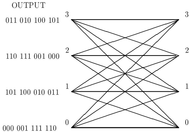
Figure 2: Trellis for Rate  $R = 2/3$ , Constraint Length 3, Non-punctured Convolutional Code.
