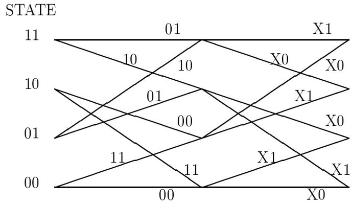
Figure 1: Trellis for Rate  $R = 1/2$ , Constraint Length 3, Period  $P = 2$  Punctured Convolutional Code.
