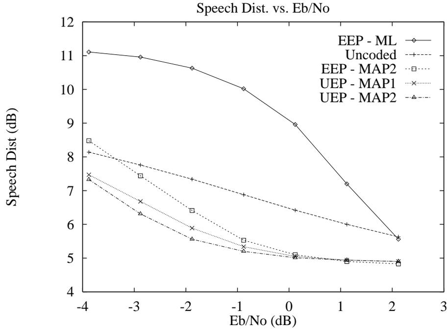
Figure 4: Average Speech Distortion for Different Coding Schemes of the LSP Parameters over the AWGN Channel.
