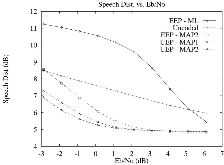
Figure 6: Average Speech Distortion for Different Coding Schemes of the LSP Parameters over the Rayleigh Fading Channel.
