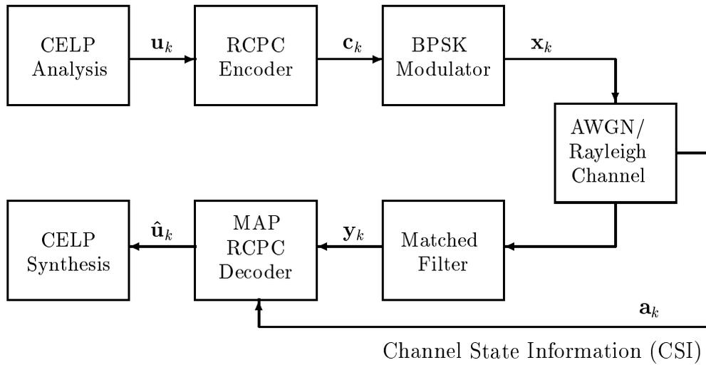
Figure 3: Block Diagram of the Overall System with MAP RCPC Decoder.
