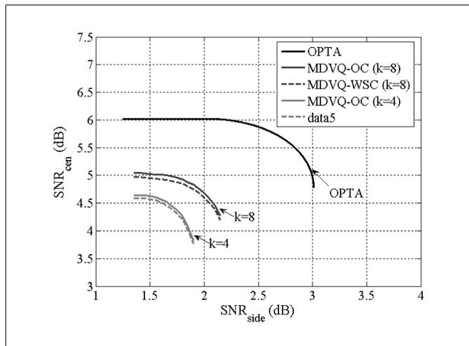
Figure 5: MDVQ for unit-variance memoryless Gaussian 4- and 8-dimensional source vectors at  $R = 0.5$  bps for various values of  $\lambda$ .
