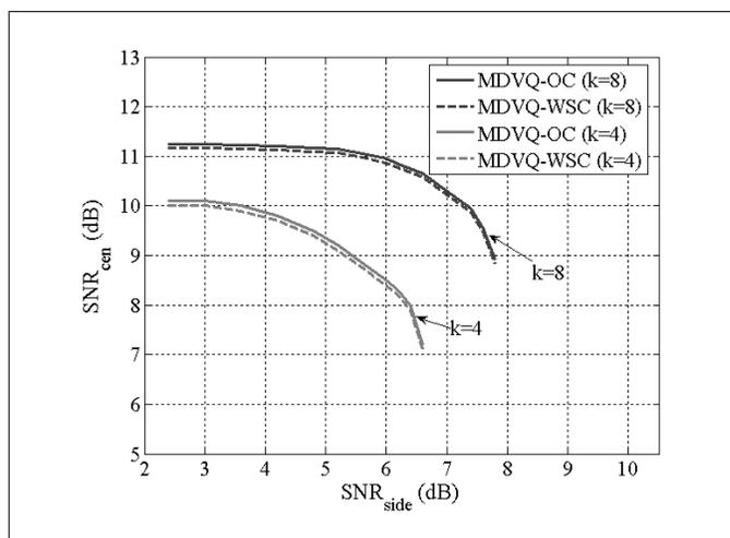
Figure 6: MDVQ for unit-variance Gauss-Markov 4- and 8-dimensional source vectors with  $\rho = 0.9$  at  $R = 0.5$  bps for various values of  $\lambda$ .
