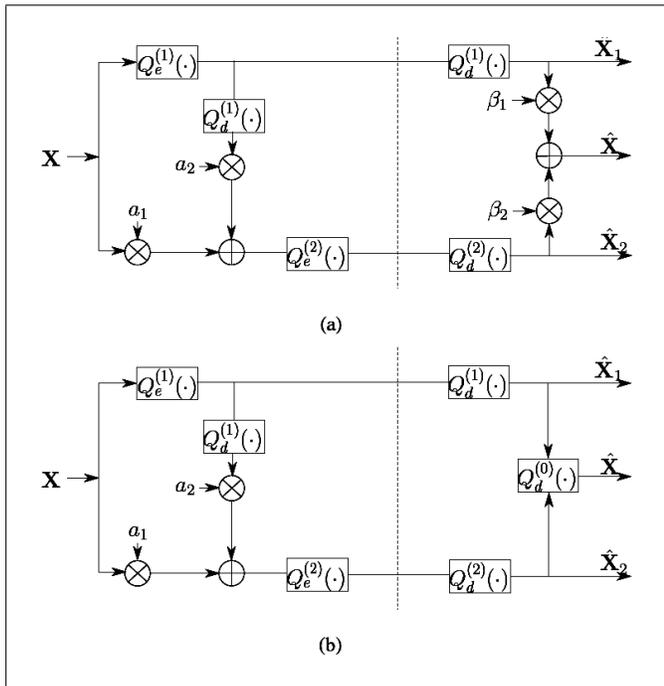
**Figure 1:** MDVQ with two channels: (a) MDVQ-WSC scheme in which the central codebook is generated as the weighted sum of the two side codebooks; (b) MDVQ-OC scheme using the optimum central decoder.
