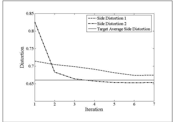
**Figure 3:** Effect of tuning the Lagrangian multipliers on side distortions for a memoryless Gaussian input source with unit variance and target side distortions  $D_{1,t} = D_{2,t} = 0.66$  ( $k = 4$  and  $R = 0.5$  bps).
