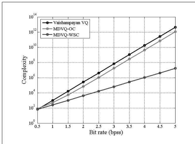
Figure 4: The complexity comparison as a function of bit rate for four-dimensional source vector.
