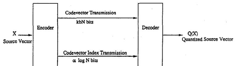
Fig. 1. Universal quantization scheme using codebook transmission.
