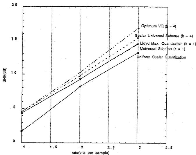
Fig. 7. Experimental performance curves for different schemes. The source is from i.i.d. zero mean, unit variance, Gaussian data truncated to  $[-2, 2]$  and  $\alpha = 50,000$ . The five curves shown from top to bottom are: (1) VQ ( $k = 4$ ) matched to the source, (2) Scalar universal scheme for VQ ( $k = 4$ ), (3) Lloyd-Max scalar quantization matched to the source, (4) Scalar universal scheme for a scalar quantizer, and (5) Uniform scalar quantization.
