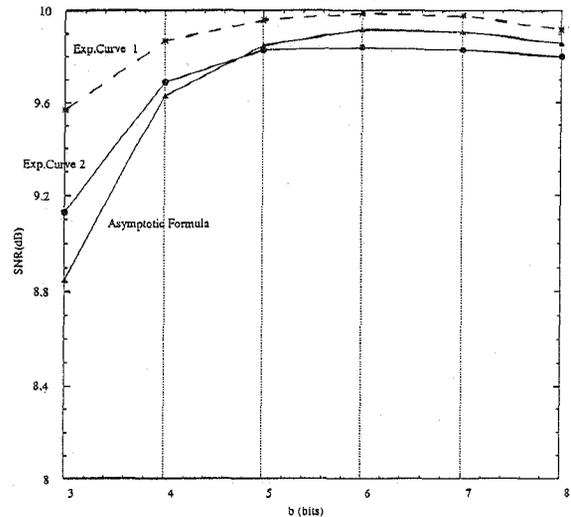
Fig. 8. Scalar universal scheme for Gaussian source, with  $k = 4$ ,  $r = 2$  bits/sample, and  $\alpha = 50,000$ . Experimental Curve 1 plots  $D(C_o)$  and Experimental Curve 2 plots  $D(C_t) + D(C_q)$ . The Asymptotic Formula curve is  $D_{opt}$ .
