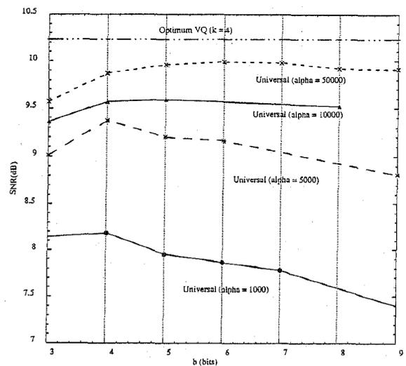
Fig. 9. Comparison of vector universal and scalar universal schemes. The source is from i.i.d. zero mean, unit variance, Gaussian data truncated to  $[-2, 2]$ ,  $k = 4$ ,  $r = 2$ . The vector universal  $C_u$  used is designed for a Laplacian.
