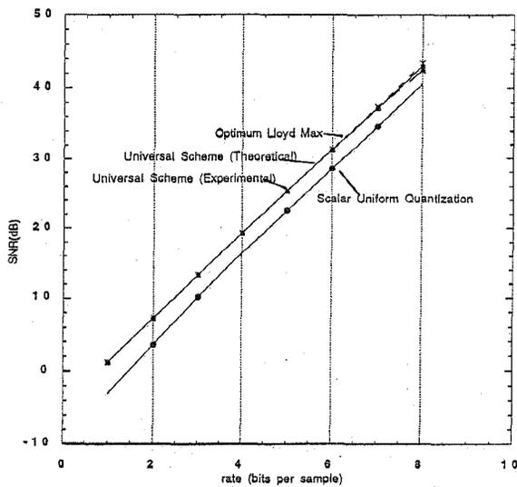
Fig. 6. Comparison of different quantization schemes. Source is from i.i.d. zero mean, unit variance, Laplacian data truncated to  $[-4, 4]$  and is scalar quantized, with  $\alpha = 50,000$ .
