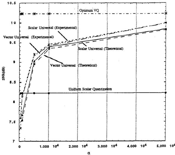
Fig. 10. Comparison of vector universal and scalar universal schemes. The source is from i.i.d. zero mean, unit variance, Gaussian data truncated to  $[-2, 2]$ ,  $kk = 4$ ,  $r = 2$ . The vector universal  $C_u$  is designed for a Laplacian.
