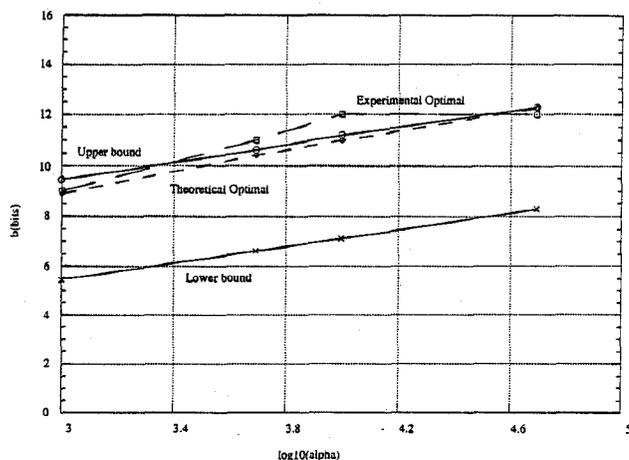
Fig. 4. Variation of  $b_{opt}$  with  $\alpha$ . Source is Laplacian truncated to  $[-4.0, 4.0]$ ,  $k = 1$  and  $r = 8$  bits/sample. The upper and lower bounds are straight lines obtained from Eq. (24) by setting  $\log_2 N = rk$  and  $\log_2 N = 0$  respectively. The Experimental curve gives the  $b$  which experimentally minimizes  $D(C_o)$ . The Theoretical curve gives the  $b$  which minimizes  $D(N, b)$  subject to  $\alpha rk = \alpha \log_2 N + kbN$ .
