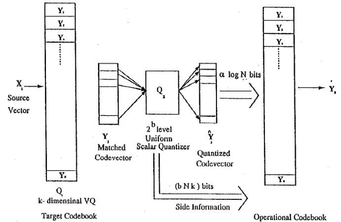
Fig. 2. Scalar universal scheme for transmission of VQ codebooks. Each component of  $\mathcal{C}_t$  is uniform scalar quantized and transmitted. The received description forms  $\mathcal{C}_o$ . Every  $\alpha$  input vectors,  $b N k$  bits are transmitted to describe  $\mathcal{C}_o$  and  $\alpha \log_2 N$  bits are sent as codevector indexes.
