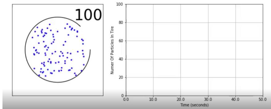
The tire animation captures the escape of molecules of air through the hole. We start with a 100 molecules with independent random positions and directions of movement, all moving at the same speed  $v$ . The students watch fascinated as the particles escape through the opening and they see the graph being plotted of the number remaining in the circle.
