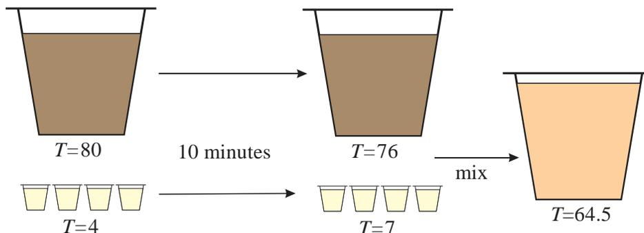
Here's the principle. If liquid 1 has temperature  $T_1$  and volume  $V_1$  and liquid 2 has temperature  $T_2$  and volume  $V_2$ , then when they are mixed the resulting temperature will be the weighted average:
