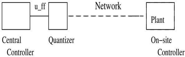
Fig. 3: Transmission of the feedforward control over the network.
