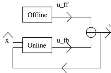
Fig. 2: Separation of the control as feedforward and feedback terms,  $\hat{x}$  denotes the estimation output.
