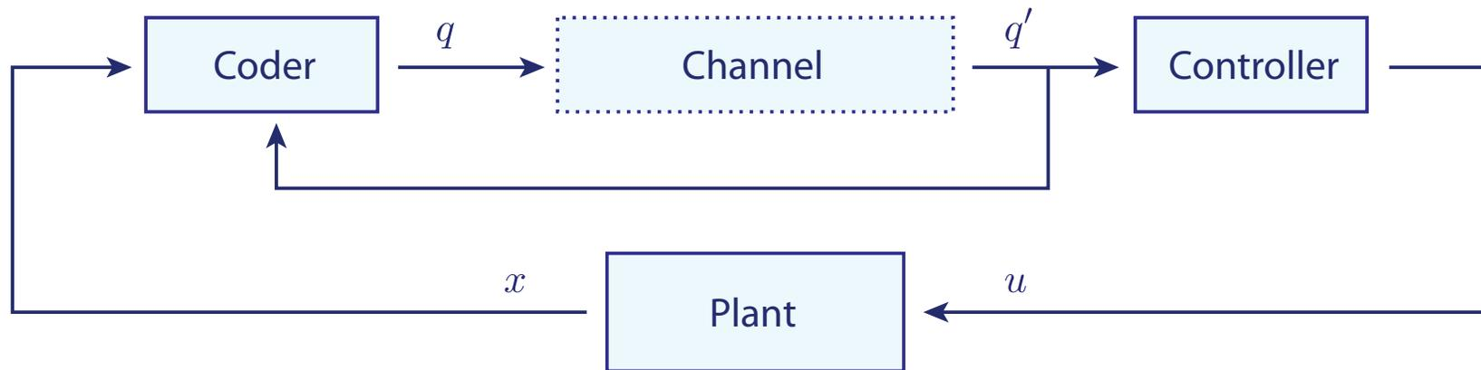
Figure 4: Control over a discrete noisy channel with feedback.
