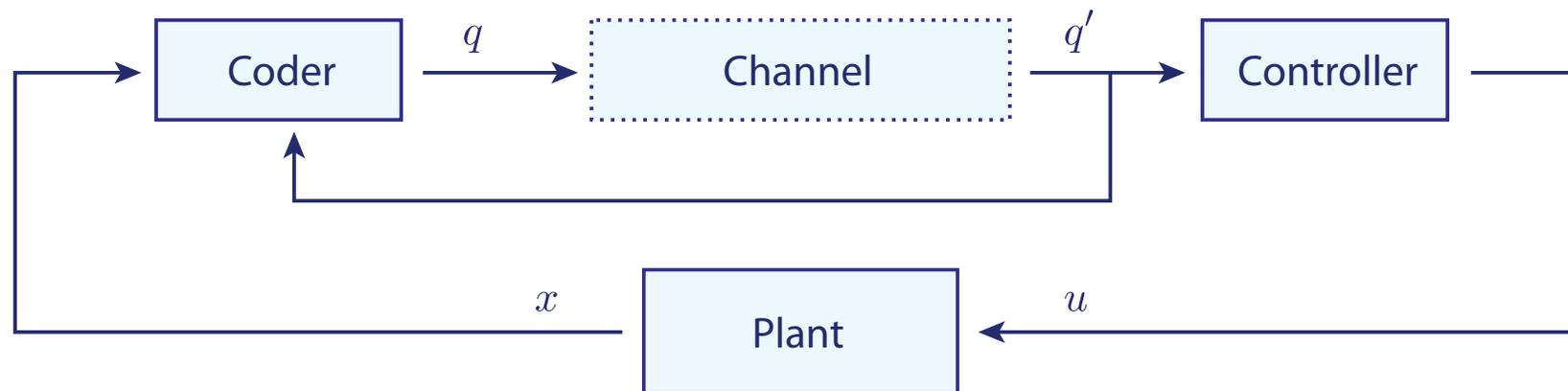
Figure 3: Encoding shapes the observation given the state. Joint design of coding and control is needed.
