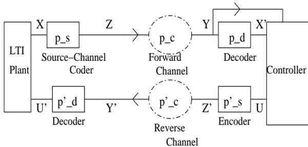
Figure 1: Control over a discrete noisy channel.
