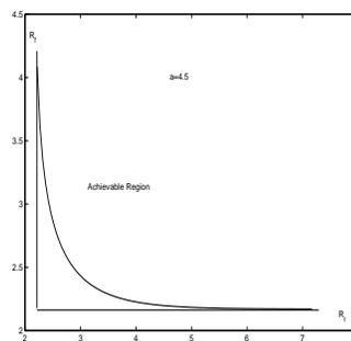
Figure 6: Forward and reverse channels trade-off for Gaussian channels. The area above the convex curve is achievable by linear memoryless policies, the areas outside the perpendicular edges are not achievable by any scheme; in the figure we have picked  $a = 4.5$ .
