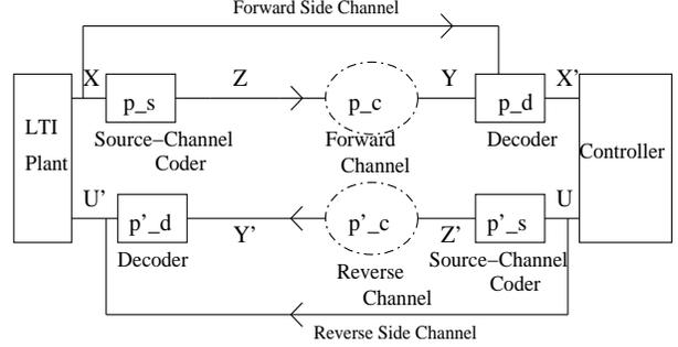
Figure 4: Side channels carry the mode of the source mapping, the system is tolerant to the errors in the side channel as well.
