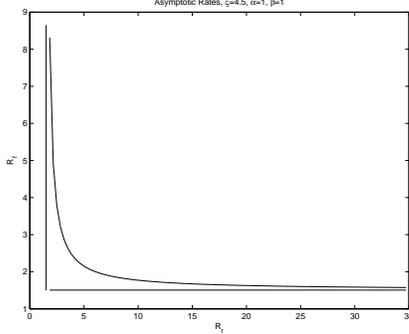
Figure 2: Achievable rates over discrete channels, the area above the curve is achievable. The area below the perpendicular lines is not achievable.
