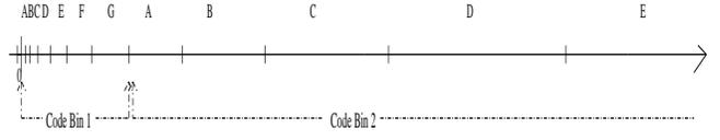
Figure 3: Illustration of the binning approach to the joint source channel code; the symbols in a given Code Bin are represented by the same channel code -letters A, B, C, ... -; the mode symbol -1,2,3 ... -is carried by the side channel.
