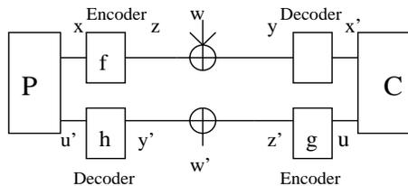
Figure 5: Control over Gaussian channels, the noise terms are  $w_f$  and  $w_r$ .
