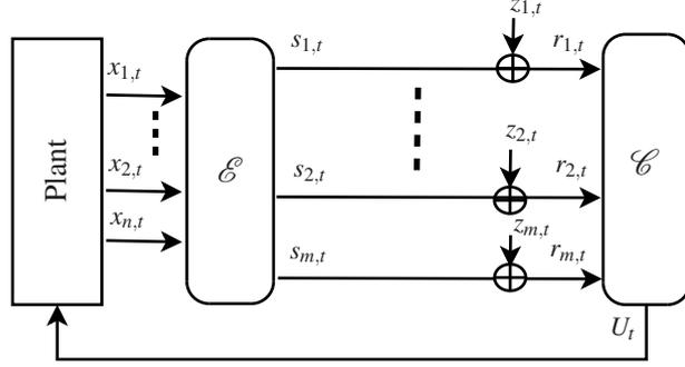
Fig. 1.2 Control over a point-point channel
