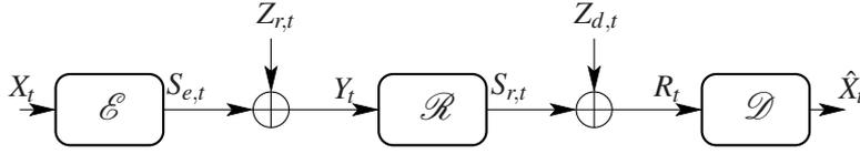
**Fig. 1.15** Real-time transmission of a memoryless Gaussian source over a two-hop relay channel.
