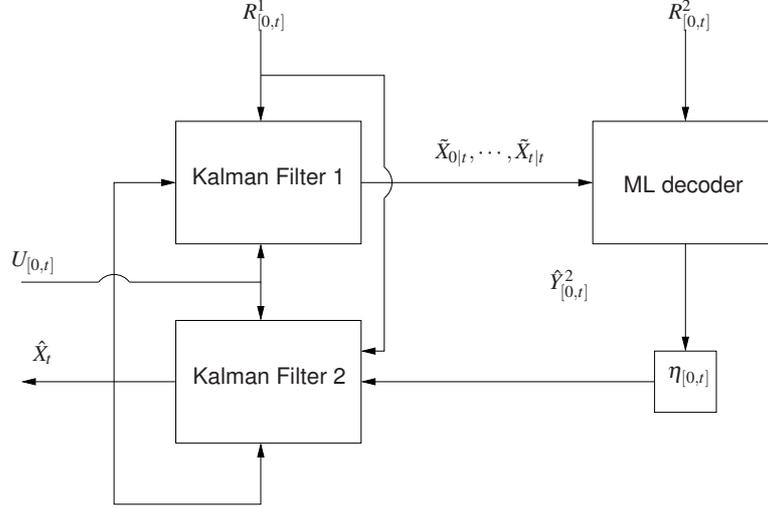
**Fig. 1.26** State estimator for the non-linear distributed sensing scheme.
