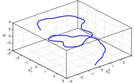
**Fig. 1.22** Relay mapping ( $K_1 = 1, K_2 = 2$ ) optimized for  $\sigma_x^2 = P_s = P_r = 1$  and  $\gamma_{ed} = 5$  dB,  $\gamma_{er} = 15$  dB, and  $\gamma_{rd} = 10$  dB.
