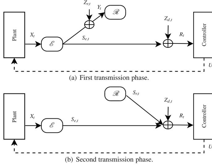
**Fig. 1.7** Half-duplex AWGN relay channel.
