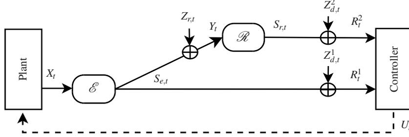
**Fig. 1.11** Orthogonal half-duplex AWGN relay channel.
