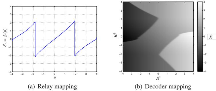
**Fig. 1.20** Relay and decoder mappings ( $K_1 = K_2 = 1$ ) optimized for  $\sigma_x^2 = P_s = P_r = 1$  and  $\gamma_{ed} = 10$  dB,  $\gamma_{er} = 10$  dB, and  $\gamma_{rd} = 25$  dB.
