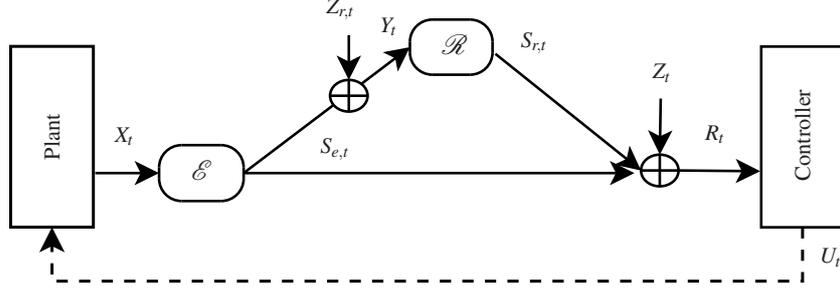
Fig. 1.10 Non-orthogonal full-duplex AWGN relay channel.
