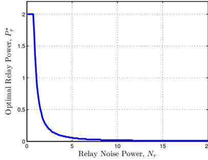
**Fig. 1.9** Optimal relay power  $P_r$  for  $P_R = 2, P_S = 10, N = 1$ .
