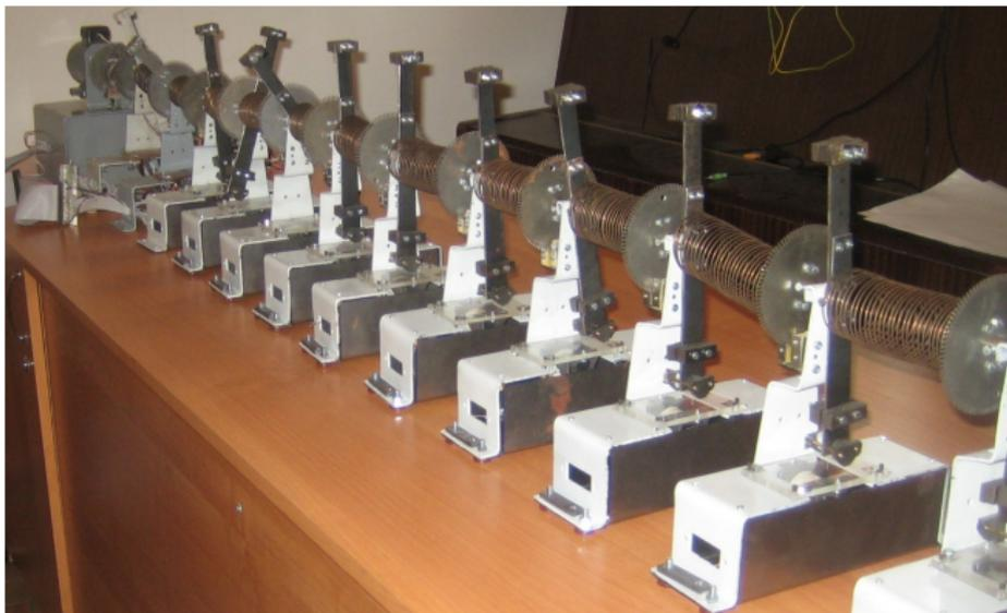
Photo of the chain of twelve pendulum sections and the motor
